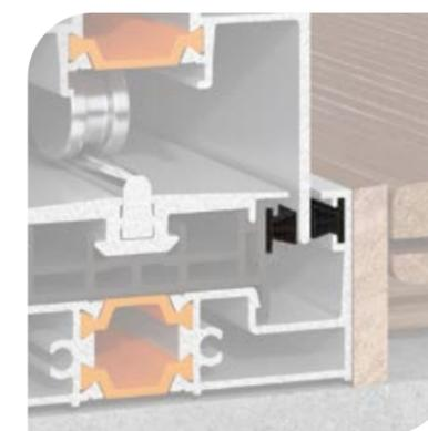
SMARTIA M630 PHOS uses **high quality brushes with triple membrane** contributing significantly to the system's air permeability and watertightness.
